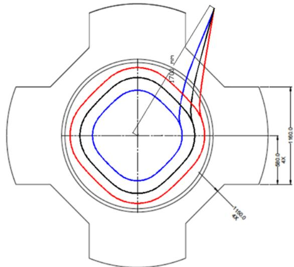
Figure 4: Equilibrium orbits and extraction trajectories for three proton beams at energies 15, 25 and 35 MeV respectively
