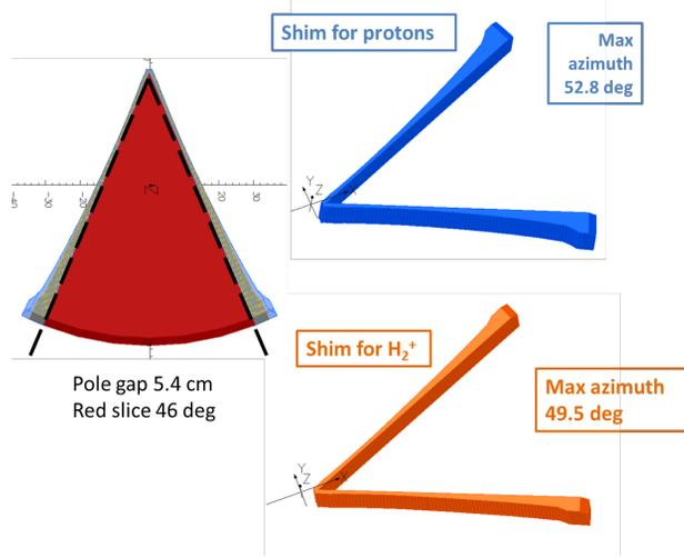
Figure 2: View of the tip of the hill and the two iron shims to adjust the field to be isochronous with  $H^-$  or  $H_2^+$  respectively.
