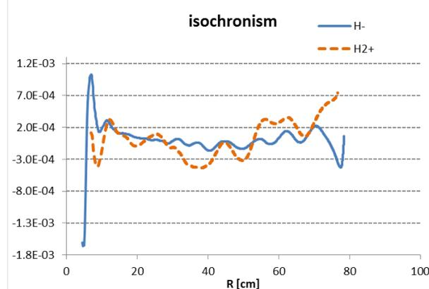
Figure 3: Ratio between the average field and the ideal isochronous field for  $H_2^+$  and  $H^-$  vs.  $R$ . The  $R$  values are not the average radius but the orbit radius at centre of the hill.
