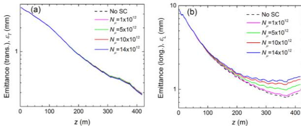
Figure 4: Emittance evolution and its dependence with the bunch charge.
