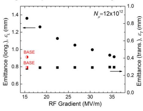
Figure 5: Final emittance achieved vs. gradient for a given space-charge intensity.
