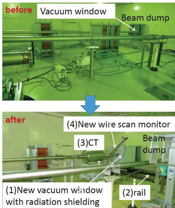
Figure 3: Pictures of beam transport line near beam dump (we call 100-deg beam dump, shown in Fig. 3(1)) before and after improvements in 2014 summer shut down.
