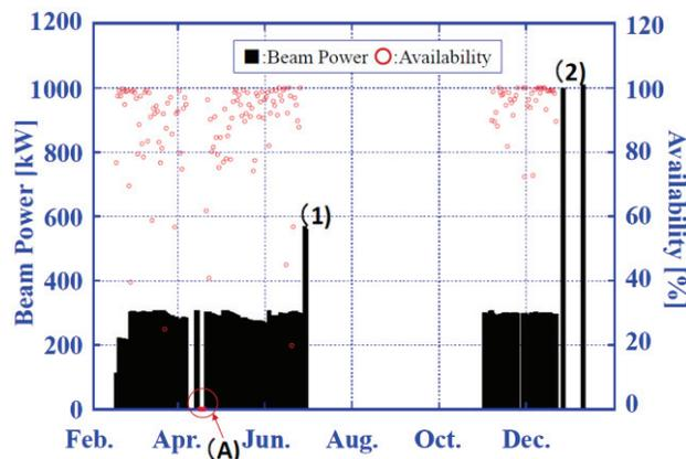
Figure 1: Output beam power and availability of the RCS from February 2014 to January 2015. Black line shows beam power and read circle shows availability. Beam studies were performed at the number (1) and (2) shown in this figure. Availability was zero at period of (A) shown in this figure due to failure of an oil cooling pump in the bending magnet choke transformer.
