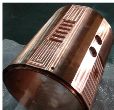
Figure 12: CH-DTL cavity wall.
