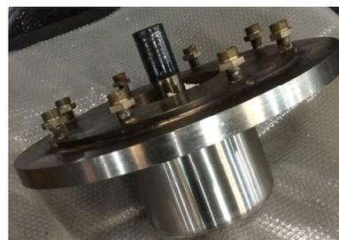
Figure 13: CH-DTL end cell.
