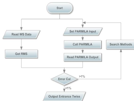
Figure 2: Algorithm Chart of Twiss Parameters Measurement Tool.
