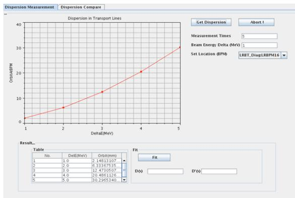
Figure 4: GUI of Dispersion Measurement Tool.
