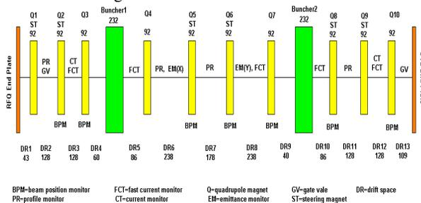
Figure 1: Schematic Drawing of CSNS MEBT.
