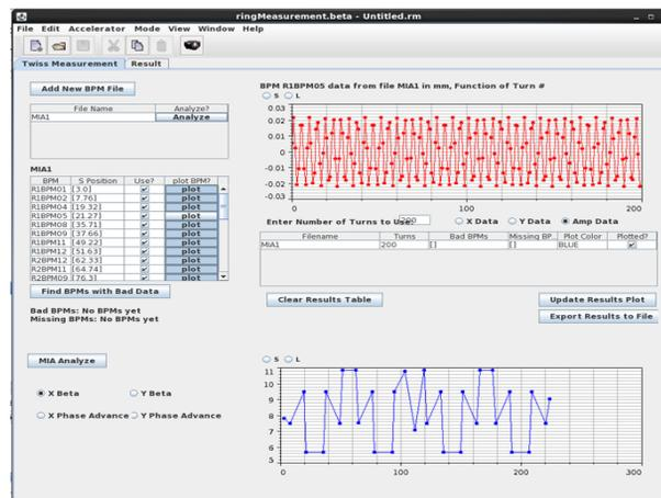
Figure 6: Beta measurement application frame.
