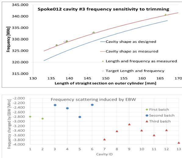
Figure 1: Frequency error caused by fabrication and EBW.
