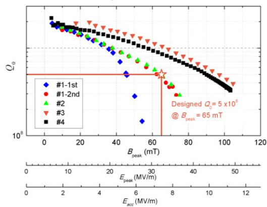
Figure 3: VT results of the spoke021 cavities.
