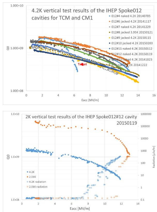
Figure 2: VT results of the spoke012 cavities.
