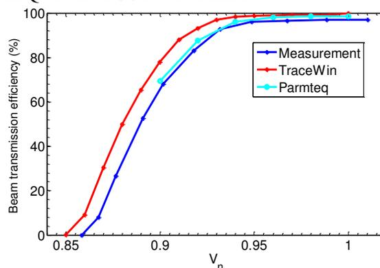
Figure 3: Measured and simulated transmissions of RFQ as functions of the inter-vane voltage  $V_n$ .
