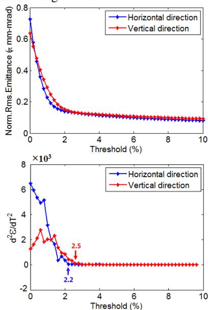
Figure 5: Emittances and the second derivative of emittance as functions of threshold of signal.
