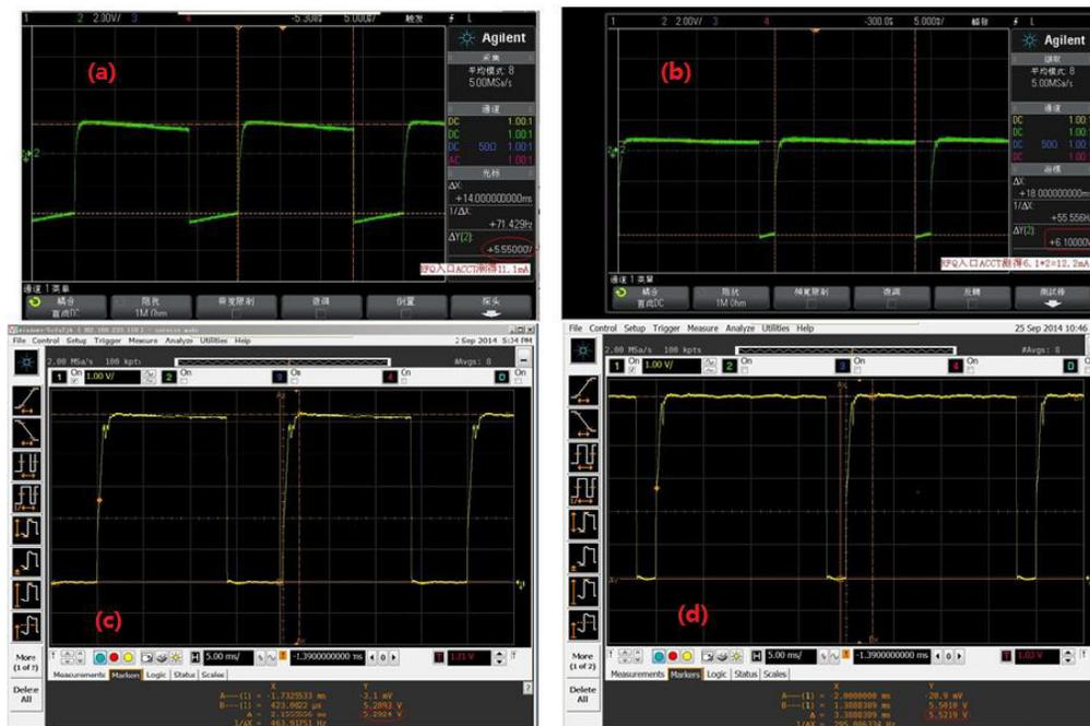
Figure 4: Beam transmission efficiency at high duty factor. (a) beam current measured by ACCT at 70% duty factor; (b) beam current measured by DCCT at 70% duty factor; (c) beam current measured by ACCT at 90% duty factor; (d) beam current measurement by DCCT at 90% duty factor.
