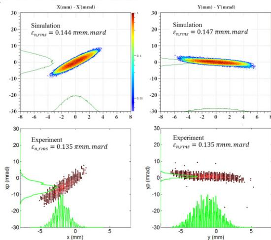
Figure 6: Simulated (upper) and measured (lower) transverse emittances and beam distribution of the RFQ.
