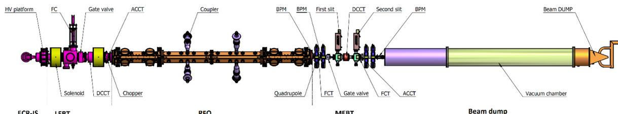
Figure 1: Layout of the test stand.
