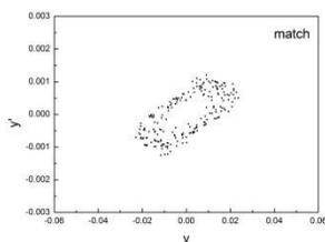
Figure 5: The position of beam-edge particles in phase space when the beam is matched.
