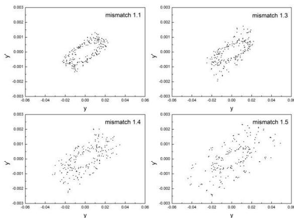
Figure 6: The position of beam-edge particles in phase space with different mismatch factor.
