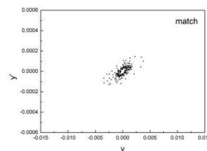
Figure 3: The position of beam-core particles in phase space when the beam is matched.
