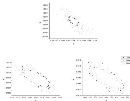
Figure 2: Up : position of particles in beam core in phase space, Bottom left: position of particles in the middle of beam in phase space, Bottom right: position of particles in the edge of beam in phase space.
