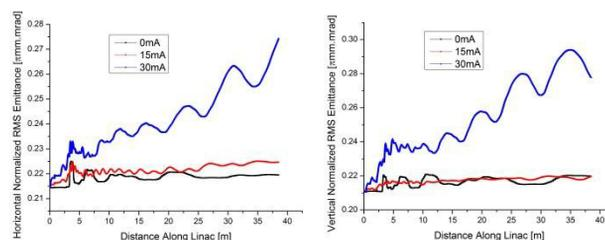
Figure 1: Left: beam horizontal RMS emittance growth along linac. Right: beam vertical RMS emittance growth along linac.
