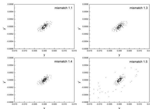
Figure 4: The position of beam-core particles in phase space with different mismatch factor.
