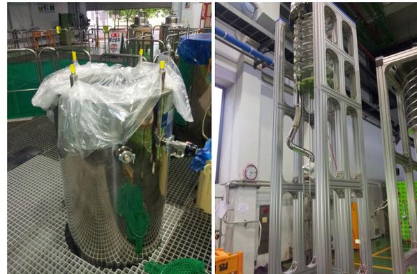
(a) Cryostat in the pit (b) Test insert in the staging rack
