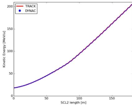
Figure 9: Energy increase through SCL2 cavities.
