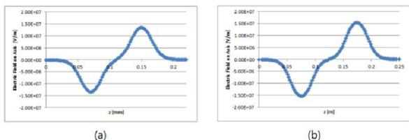
Figure 4: Field profile on beam axis for (a) QWR and (b) HWR cavities.
