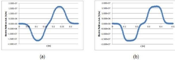
Figure 8: Field profile on beam axis for (a) SSR1 and (b) SSR2 cavities.
