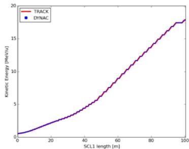
Figure 5: Energy increase through SCL1 cavities.
