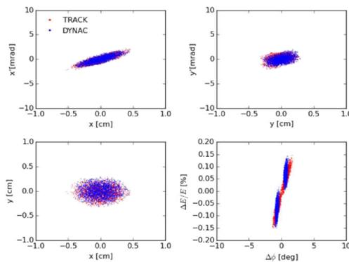
Figure 7: Particle distributions in  $x-x'$ ,  $y-y'$ ,  $x-y$ , and  $\Delta\phi-\Delta W/W$  spaces at the end of SCL1.
