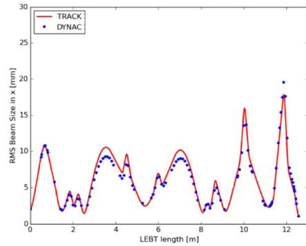
Figure 2: The rms beam envelope through RAON LEBT by DYNAC and TRACK codes.
