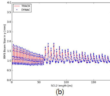
Figure 11: The rms envelop through SCL2 cavities in (a) horizontal and (b) vertical directions.
