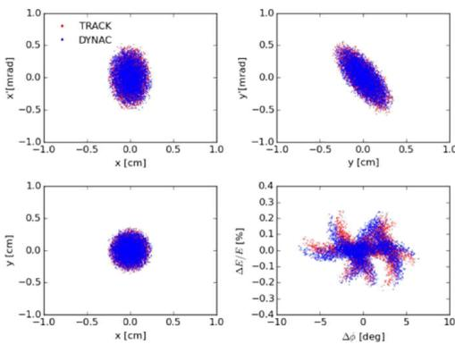
Figure 10: Particle distributions in  $x-x'$ ,  $y-y'$ ,  $x-y$ , and  $\Delta\phi-\Delta W/W$  spaces at the end of SCL2.
