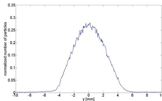
Figure 6: Vertical measured profile after shaving at 160 MeV. The  $1\sigma$  beam profile was calculated to be 2.25 mm, giving a normalized emittance of  $0.8 \mu\text{m}$ .
