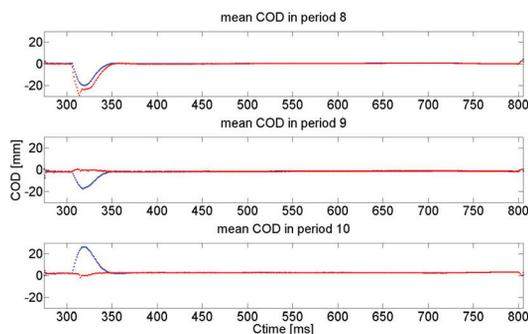
Figure 5: Measured COD in period 8, 9 and 10 for the two shaving methods: conventional one marked in blue and new, studied method, using a closed bump in red.
