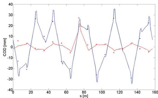
Figure 2: Simulated (continuous line) and measured (points) vertical closed orbit distortion in the machine. The operational shaving is marked in blue colour and the proposed new shaving scheme in red colour.
