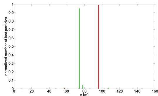
Figure 3: Simulated losses in the machine at 63 MeV for the current situation (red colour) and the proposed new shaving scheme (green colour).
