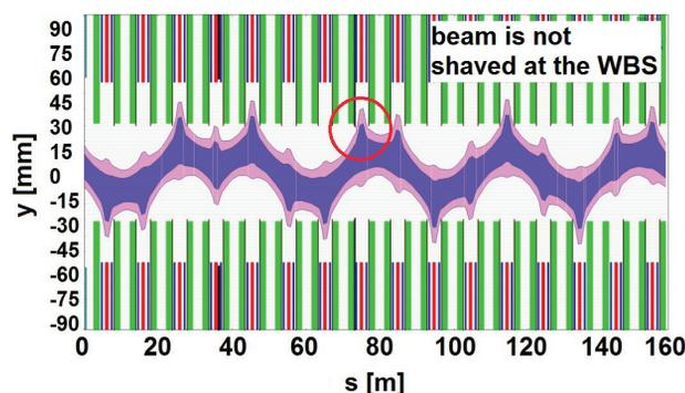
Figure 1: Lattice of the PSB and the illustration of the 3 sigma beam while conventional shaving. The 3-sigma beam is plotted in violet while 5 sigma is in magenta. The beam envelope is calculated for the vertical plane, with  $Q_x = 4.37$  and  $Q_y = 4.45$ . Main lattice elements are shown in different colours: bending magnets in green, focusing quadrupoles in blue and defocusing quadrupoles in red. The scrapers are marked in maroon and WBS with the red circle.
