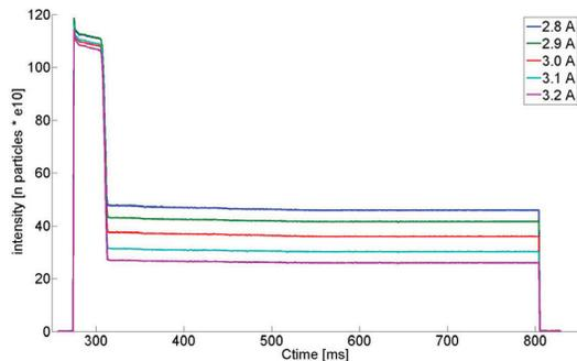
Figure 4: Intensity versus time in the cycle for different shaving currents set on DBSV7 and DBSV9.
