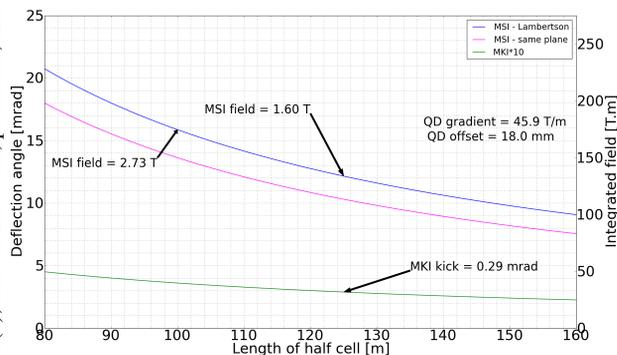
Figure 3: Kick angle and integrated field of septum (MSI) and kicker (MKI) as a function of the half cell length.
