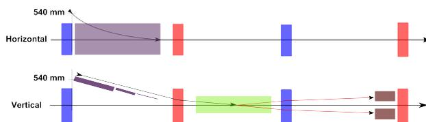
Figure 2: Layout of the injection system. Focussing (red) and defocussing (blue) quadrupoles build a FODO lattice. The Lambertson septum (violet), which is vertically aligned with the incoming trajectory angle, deflects the beam horizontally onto the orbit, and the kicker (green) compensates for the remaining angle in the vertical plane. The injection dump (brown) intercepts miskicked beam (red).
