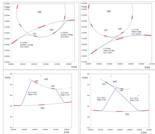
Figure 4: Transfer line geometries between LHC and FCC (left) for the intersecting option in horizontal (top) and vertical (bottom) planes and (right) for the non-intersecting option.
