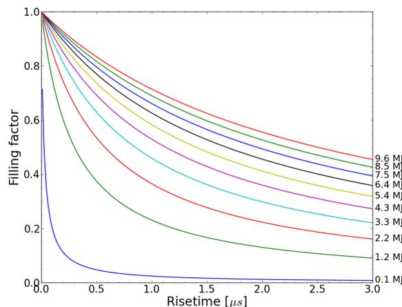
Figure 1: FCC bunch fill factor vs injection kickers rise time for different transferred beam energies. The foreseen filling of 80% is reached for HL-LHC energies (about 5 MJ) for a rise time of 0.28  $\mu\text{s}$ .
