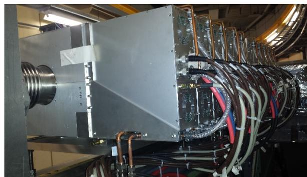
Figure 1: Prototype Finemet cavity modules installed in Ring 4 of the PSB.
