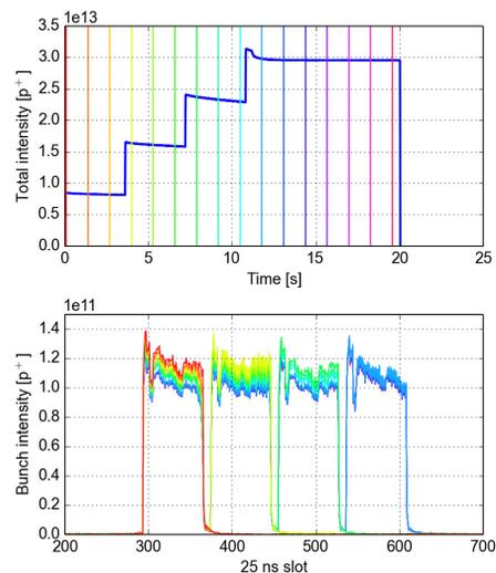
Figure 2: Four batches of 25 ns beam injected and accelerated to 450 GeV with 'acceptable' beam losses. The lower plot shows the snapshots of the bunch-by-bunch intensity taken at the cuts shown in the above plot.
