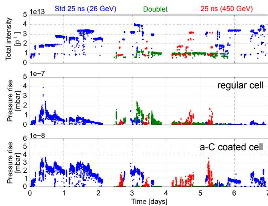
Figure 1: Week 45: Cycle-by-cycle maximum injected intensity in the SPS in protons (top), dynamic pressure rise in a regular cell (middle), dynamic pressure rise in an a-C coated cell (bottom).
