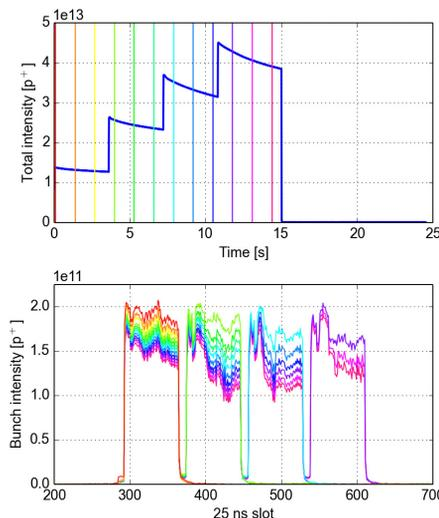
Figure 4: Four batches of high intensity 25 ns beam with large beam losses. The lower plot shows the snapshots of the bunch-by-bunch intensity taken at the cuts shown in the above plot.
