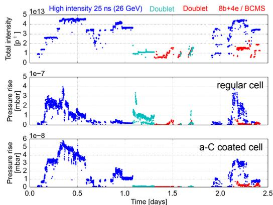
Figure 3: Week 50: Cycle-by-cycle maximum injected intensity in the SPS in protons (top), dynamic pressure rise in a regular cell (middle), dynamic pressure rise in an a-C coated cell (bottom).
