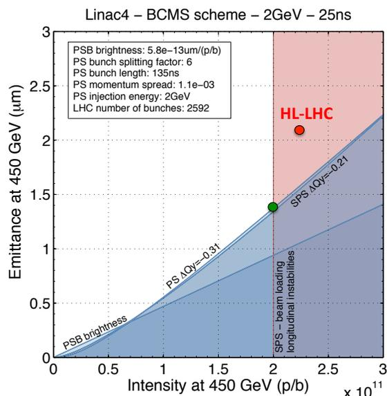
Figure 3: Proton performance reach with BCMS beams.
