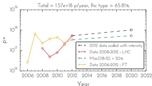
Figure 1: Extrapolation of the expected intensity to be dumped per year for post-LS2 era based on available data.
