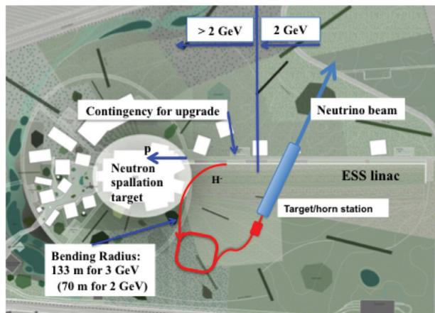
Figure 2: The accumulator on the ESS site.
