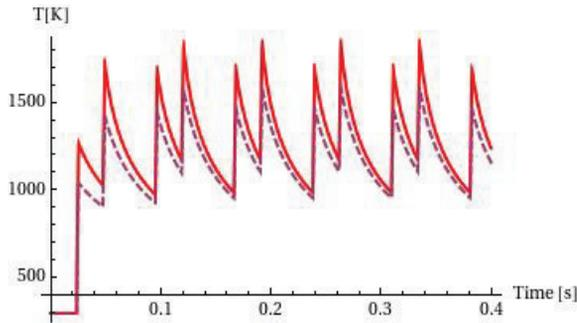
Figure 3: Evolution of maximum foil temperatures [K] at the H<sup>-</sup> - spot peak (dashed) and the combined H<sup>-</sup> and circulating protons peak (red). Only two injections into the accumulator per linac pulse.
