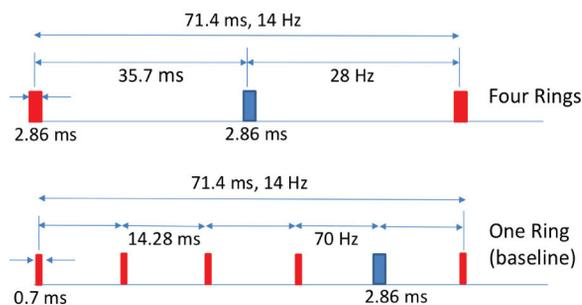
Figure 1: Pulse distribution for the 4-ring and the one-ring options: The upper part of the figure shows the 28 Hz pulsing of the linac with one proton (blue) and one H<sup>-</sup> (red) pulse interleaved and the lower part shows the case where four 0.72 ms long pulses of H<sup>-</sup> for neutrinos are followed by one 2.86 ms proton pulse for the neutrino spallation target.
