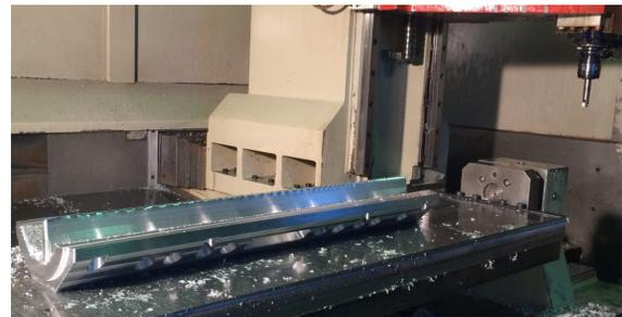
Figure 6: Test machining of the RFQ vane.
