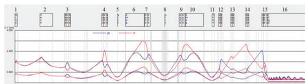
Figure 3: Beam envelopes during the transport from the EBIS-CB platform to the ATLAS RFQ. 1 - einzel lens; 2 - acceleration to 30.6keV/u; 3,4,15 - electrostatic triplets; 5,8 - slits ; 6,10 - 90° dipoles; 7,9,12-14 - electrostatic doublets; 10 - MHB; 16-ATLAS RFQ.
