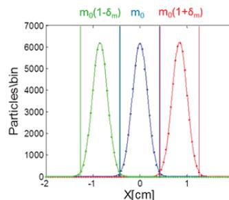
Figure 4: Beam profiles at the mass selection slit,  $\delta_m=6.7\cdot 10^{-3}$ . Vertical lines indicate intervals containing 99% of the particles in each distribution.
