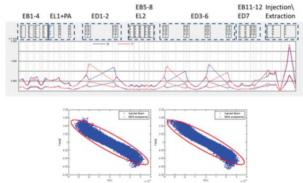
Figure 6: Top: beam envelopes during the beam transport from the MR-TOF exit to the EBIS-CB. Bottom: phase space projections of the beam at injection to EBIS-CB.
