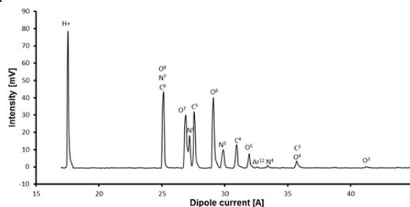
Figure 1: Residual gas spectrum after 30ms breeding.
