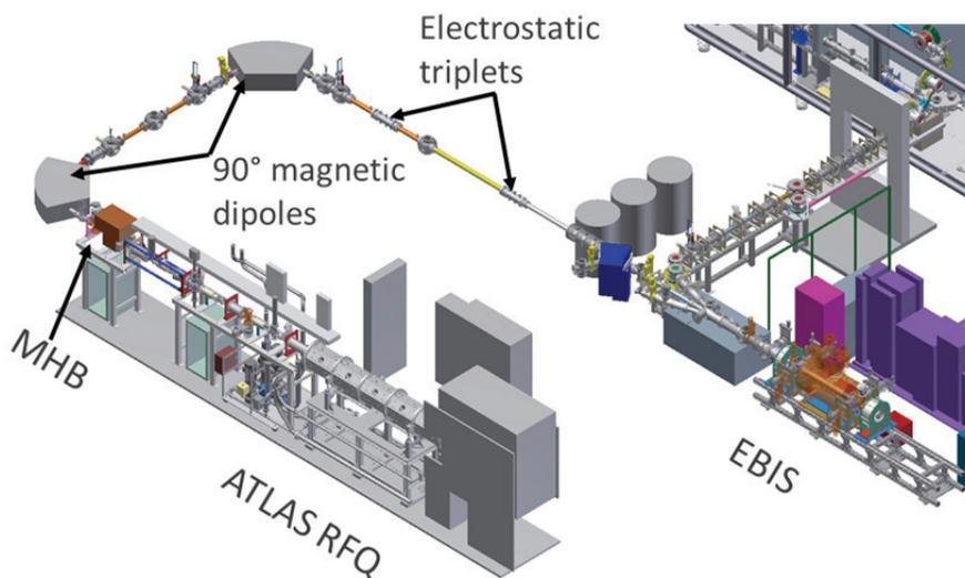
Figure 2: A 3d model of the low energy beam transport line from the EBIS-CB platform to the ATLAS RFQ.
