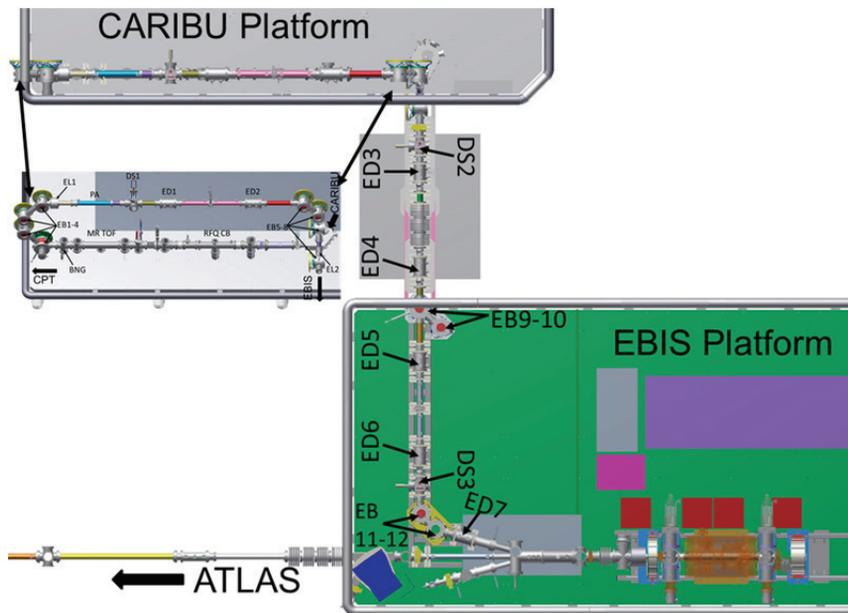
Figure 5: A 3d model of the transport line from CARIBU to the EBIS-CB: EB1-12 – spherical electrostatic benders; ED1-7 – electrostatic doublets; EL1-2 einzel lenses; PA – pulsed accelerator; MR-TOF – Multi Reflection Time of Flight spectrometer;
