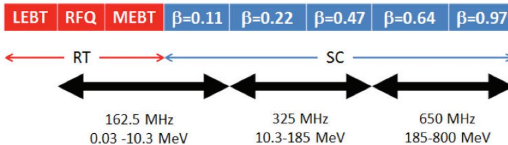
Figure 2: The SC Linac technology map. Items in red are at room temperature, items in blue are superconducting.  $\beta$  values represent the optimal values for each cavity type.
