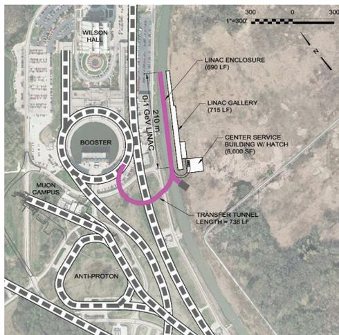
Figure 1: Site layout of PIP-II. New construction is predominantly in the Tevatron infield. Grey dashed areas represent existing underground enclosures.
