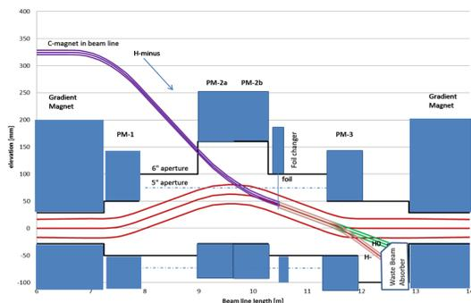
Figure 3: Initial concept for PIP-II injection into Booster.
