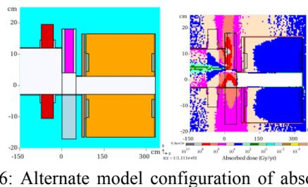
Figure 6: Alternate model configuration of absorber and adjacent magnets(left) and absorbed dose (right).
