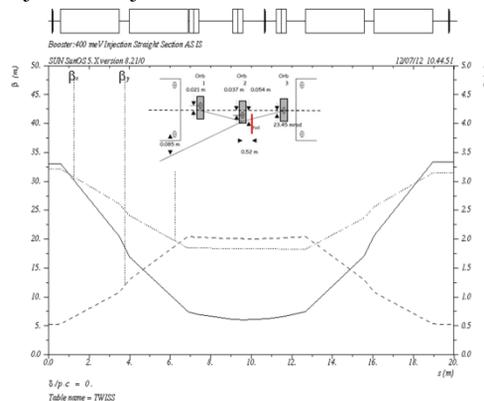
Figure 2: Current Booster injection straight section lattice.
