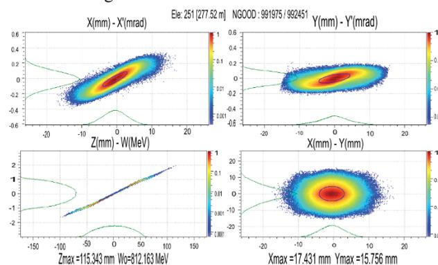
Figure 6: Output distribution of the Transfer Line tracking simulation with TraceWin.
