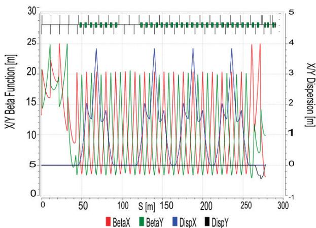
Figure 2: Optics of the Transfer Line (baseline).
