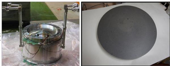
Figure 5: (a) LH<sub>2</sub> absorber (left) and (b) LiH disk (right).
