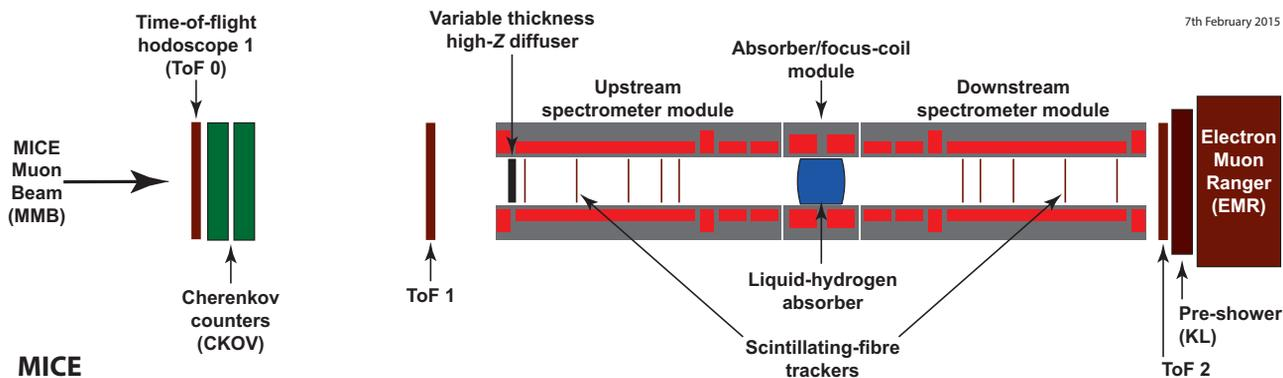
Figure 1: Schematic layout of MICE Step IV.
