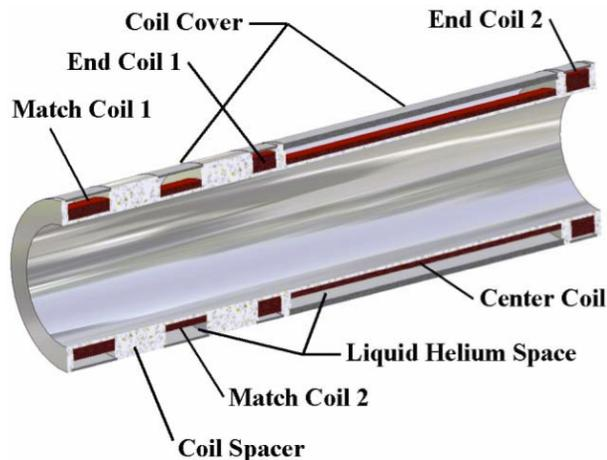
Figure 2: Cross section of a spectrometer solenoid magnet.
