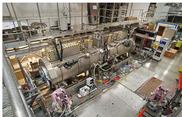
Figure 3: MICE spectrometer solenoids magnets installed in the MICE Hall. The AFC module can be seen situated between the two solenoid modules.
