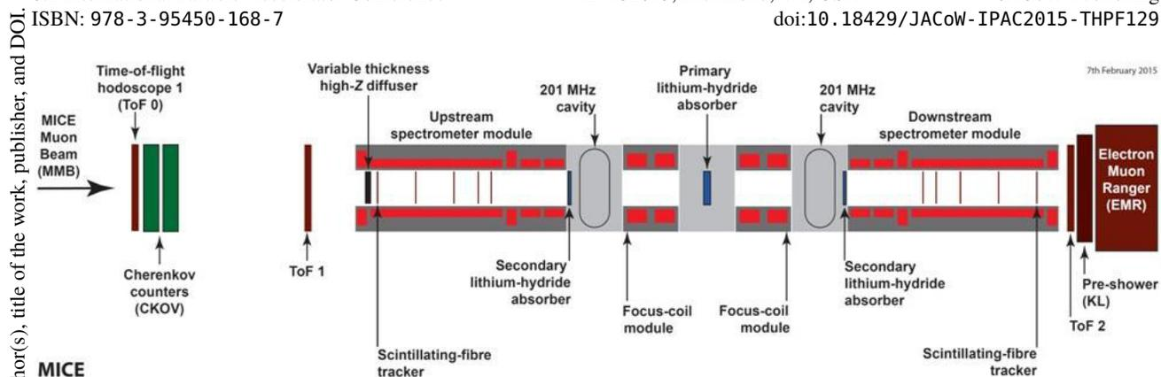
Figure 1: Layout of the novel lattice configuration for the MICE Cooling Demonstration.
