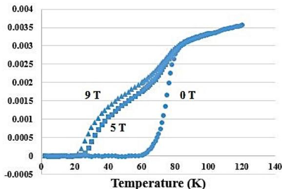
Figure 5: Resistance measurement of ETP pellet at 0 T, 5 T, and 9 T.
