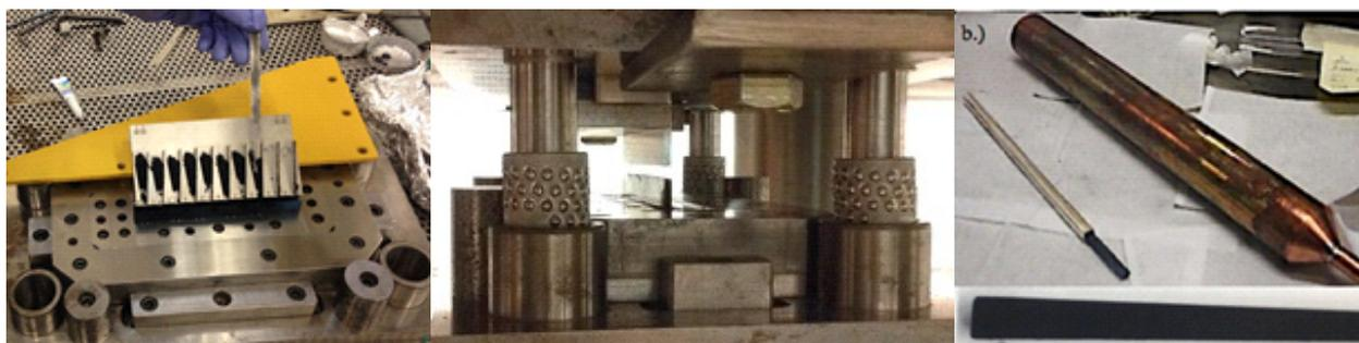
Figure 1: Fabrication of square-cross-section textured-powder Bi-2212 core a) load fine-powder Bi-2212 into rectangular die in oxygen atmosphere; b) compress to 200 MPa; insert bar into square hole in silver tube.
