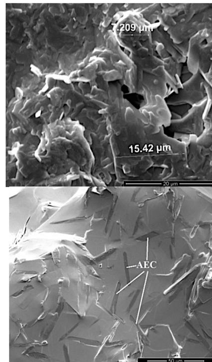
Figure 3: a)  $T_{max} = 878$  C, not melted; b)  $T_{max} = 881$  C, melted.
