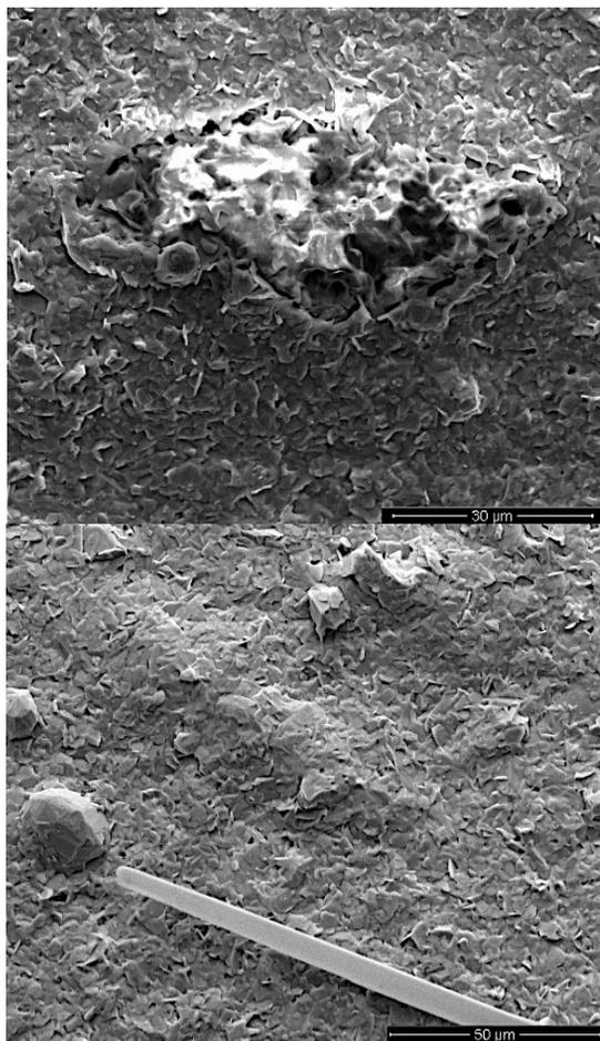
Figure 4: ETP cores heat treated at  $T_{max} = 876$  C: a) no annealing, parasitic phase visible; b) annealed, phase-pure Bi-2212.
