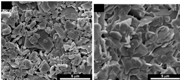
Figure 2: SEM micrographs of TP cores before and after non-melt heat treatment at 879 C for 2 hours.
