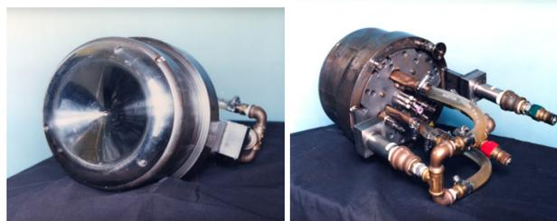
Figure 1: Side view of assembled LANSCE duoplasmatron ion source with Pierce electrode.
