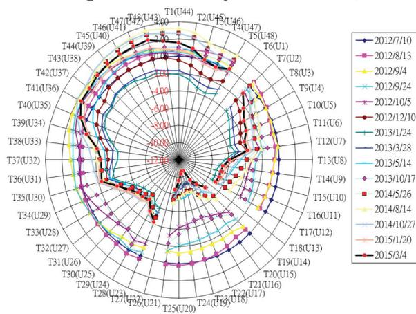
Figure 11: The TPS building variation in radius direction.
