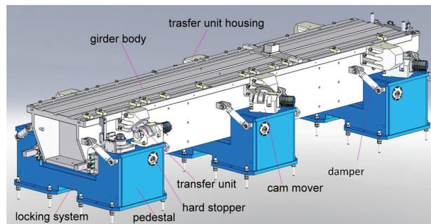
Figure 4: One girder configuration.
