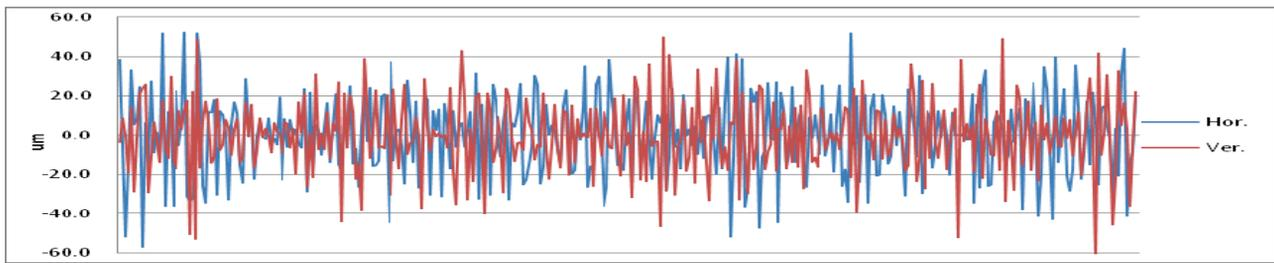
Figure 14: The position deviations of each magnet center when assembled on the girder.
