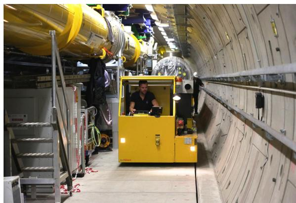
Figure 2: Cryomodule transport into the XFEL tunnel.
