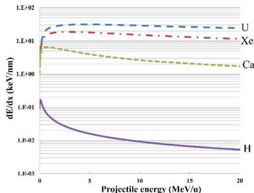
Figure 1: Comparison of the energy loss per unit length in carbon foils for some heavy ions and protons. A single U ion deposits three orders of magnitude higher power than a proton of the same velocity. Stripping energies at FRIB are between 16 and 20 MeV/u.
