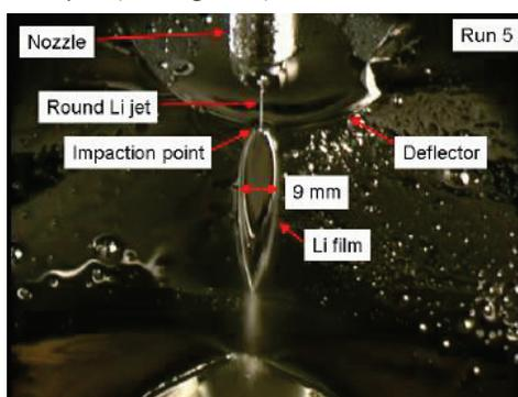
Figure 2: Liquid lithium film formed by impact of a high velocity jet on a deflector at the ANL lithium test stand [6].
