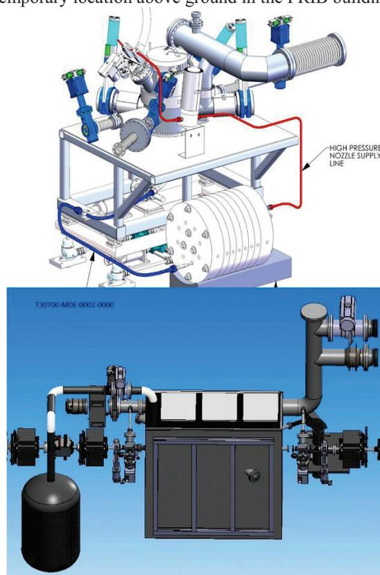
Figure 6: Top: The components of the liquid lithium stripper are shown. The pump is in the forefront. Bottom: we show the steel secondary containment vessel (2 m long) that will remain full of Ar. A vent to a scrubber is shown on the upper right and the Ar supply tank on the lower left.
