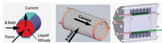
Figure 4: Electromagnetic pump developed for liquid lithium. The current ( $\sim 2000$  A) is axial in the helical coil while the magnetic field ( $\sim 6$  kG, generated by permanent magnets) is radial. The force on the lithium is in the azimuthal direction. The gray squares in the cross section show the permanent magnets.
