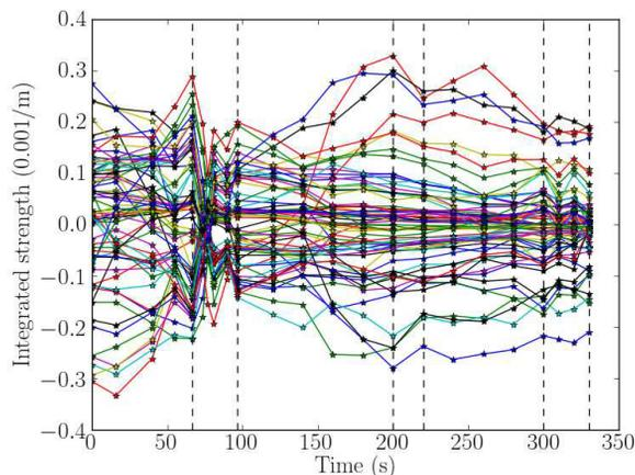
Figure 3: The calculated correction strength for the 72 trim quadrupoles in the Yellow ring on the energy ramp, the dashed lines are at the step-stones where settings for quadrupoles (some or all) are fixed. The horizontal axis is the time in seconds from the time the acceleration ramp starts.
