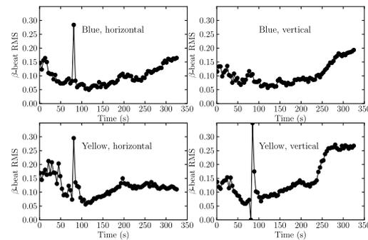
Figure 1: The measured beta-beats during beam acceleration (high energy Au-Au, 2014). Transition crossing occurs at  $\sim 85$  seconds after the start of acceleration.
