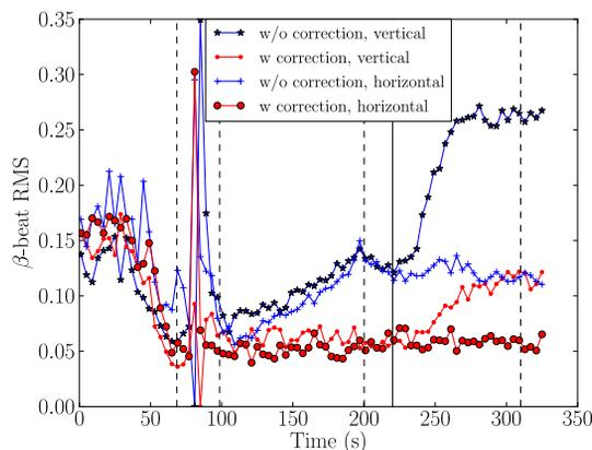
Figure 4: The measured global RMS beta-beats in the Yellow ring with (w) and without (w/o) ramp optics corrections. Optics corrections were implemented at 6 intermediate energies, at the times indicated by the vertical lines, with linear interpolation in-between.
