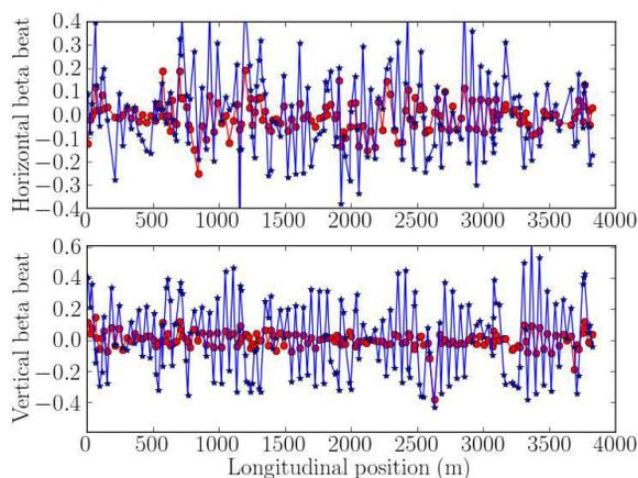
Figure 2: The beta-beats before and after optics correction in the Yellow ring for low energy run in 2014: the upper and lower plot show the horizontal and vertical beta-beats. The blue data point is the beta-beat before the corrections and red is after the corrections.
