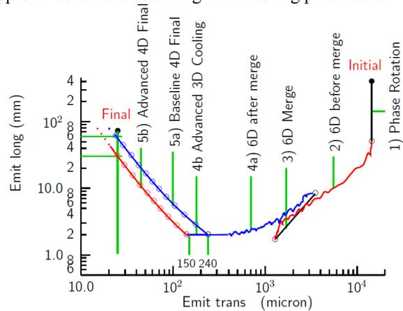
Figure 1: Progression of emittances throughout a collider cooling scenario.
