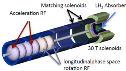
Figure 2: A cell of final cooling.
