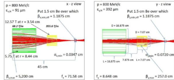
Figure 3:  $\mu$  trajectories (x and y) through a quad doublet for a  $\beta^* = 1cm$ . cooling channel.
