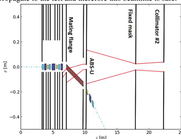
Figure 1: Example of particle tracking for SRX beamline. Tracking starts at Collimator #2 on the right and attempts to get to the storage ring straight on the left. The red lines denote the envelope of trajectories. No trajectories pass to the straight, therefore these are safe.
