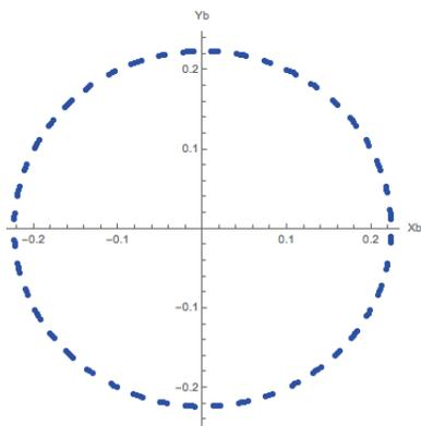
Figure 2: Particle positions calculated at the end of each period of function  $g$  ( $s=0, 2, 4, \dots$ ) for 300 periods. One dot corresponds to one position. The magnitude of  $g$  is such that  $\theta=1/4$  rad (value chosen for illustration only). For other choices of initial position  $s$  the  $(x,y)$  locations follow an ellipse.
