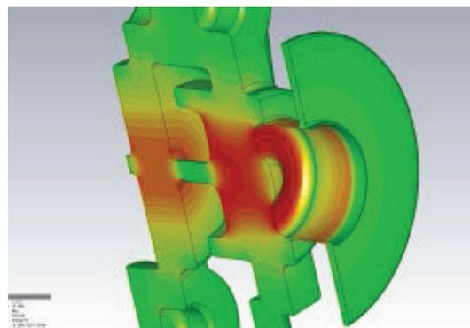
Figure 7: Choke structure of cathode rod.
