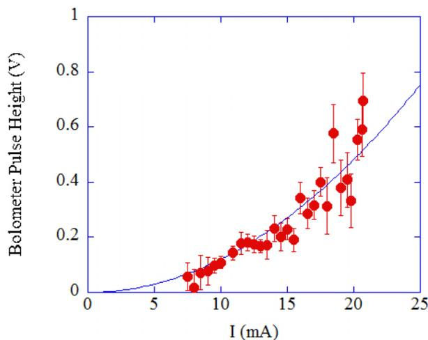
Figure 2: Edge radiation intensity as a function of beam current. The solid line is a quadratic curve obtained by fitting the data.
