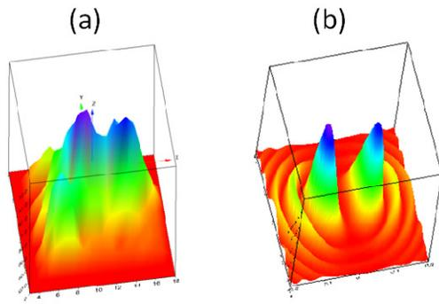
Figure 4: Spatial distribution of horizontal polarized component of edge radiation: (a) experiment (b) calculation.
