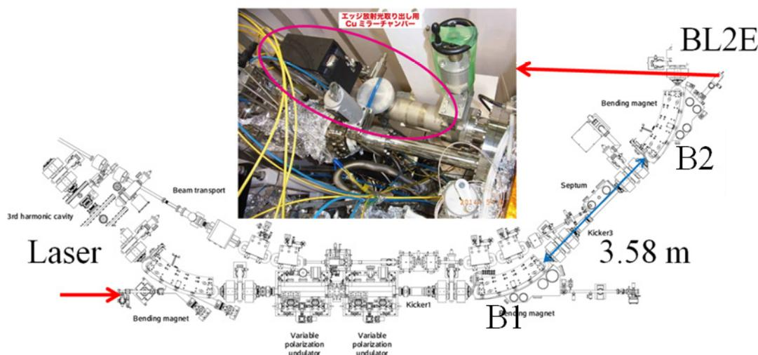
Figure 1: Drawing of UVSOR-III storage ring around undulator 1U [6] and a photograph of BL2E beam-line for detection of edge radiation.
