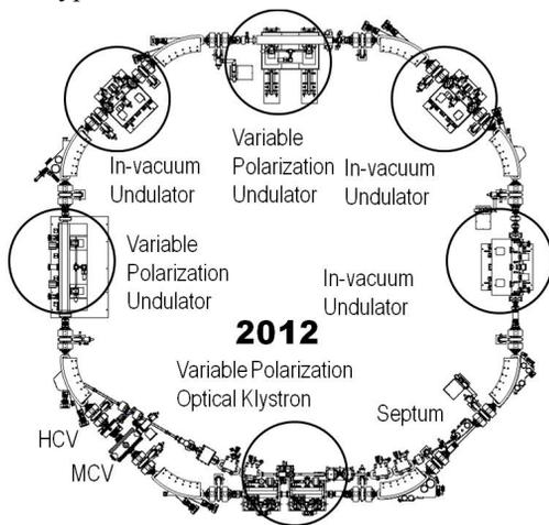
Figure 2: Configuration of UVSOR-III [24].
