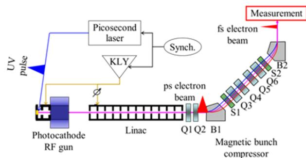
Figure 1: Diagram of photocathode-based linac.
