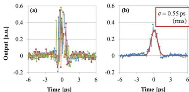
Figure 4: Temporal electric field profiles of (a) three sequential sweeps and (b) averaged data using twelve sweeps.
