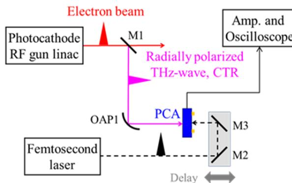
Figure 3: Schematic diagram of time-domain measurement of CTR using the PCA.
