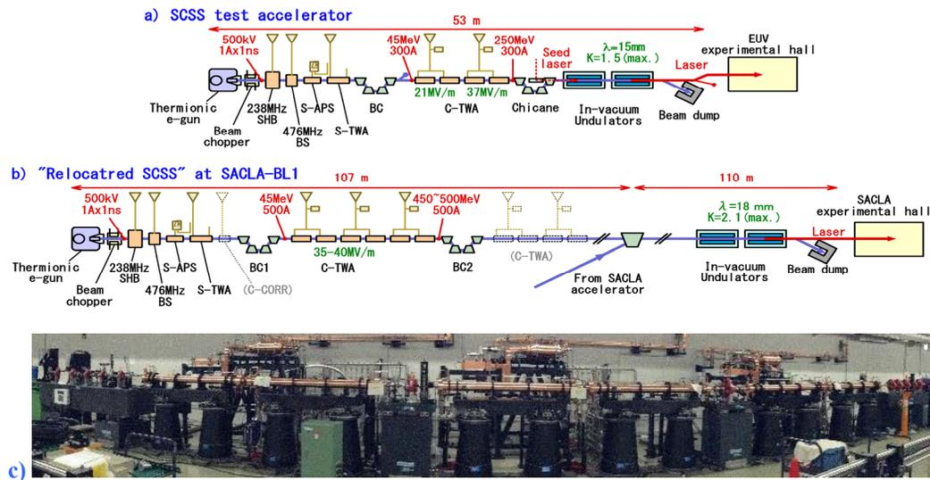
Figure 2: Machine configurations of a) the SCSS test accelerator, b) the relocated SCSS machine and c) installed machine situation in the SACLA undulator hall [5].
