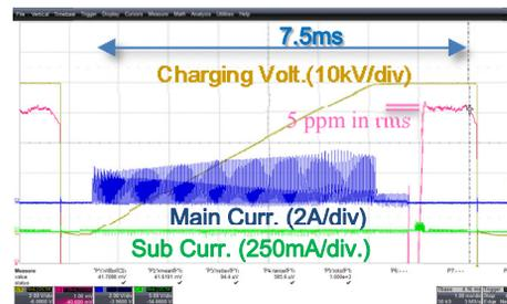
Figure 6: Output wave forms of the high-precision inverter charger. The charging voltage is 50 kV. [8]
