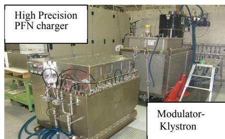
Figure 5: Outlook of the high-precision inverter charger for the PFN of the klystron modulator. [4,8]
