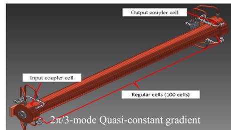
Figure 3: Outlook of the accelerating structure. [6]
