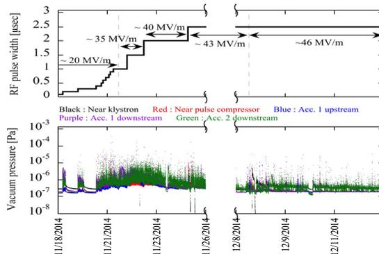
Figure 7: High-power rf conditioning history of the C-band accelerating structures (CB1-1). The rf pulse width and power were increased during 24 days.
