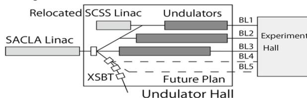
Figure 1: Place to install the relocated SCSS test accelerator (LINAC) in the undulator hall of SACLA.
