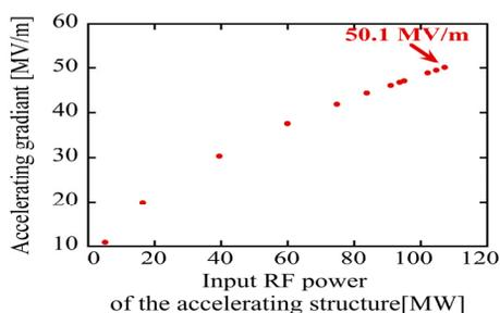
Figure 4: Acceleration gradients of the  $2\pi/3$  CG accelerating structure, as a function of its input rf powers. These gradients are calculated by using an averaged shunt impedance of  $64 \text{ M}\Omega/\text{m}$ . [4,6]
