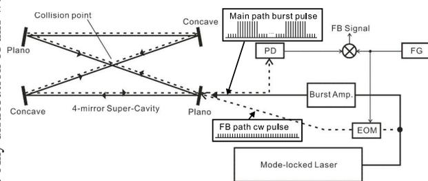
Figure 2: Schematic of burst mode optical enhancement cavity.
