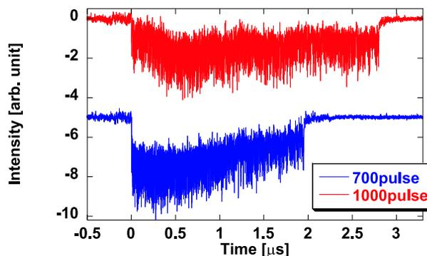
Figure 3: 700 and 1000 pulse X-ray train detected by MCP.
