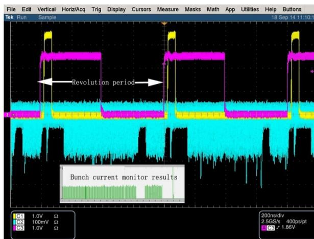
Figure 2: Gate signals used for synchronization with the camshaft pulse. The oscilloscope is working in the infinite remainder seen mode.
