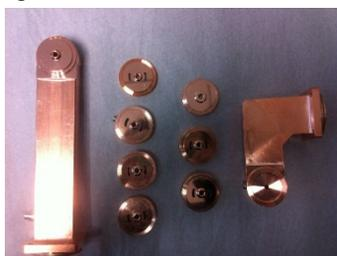
Figure 3: Machined cells of accelerator tube.
