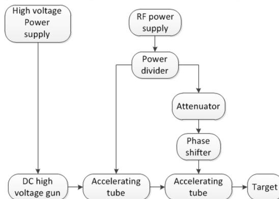
Figure 1: Schematic diagram of the linac system.
