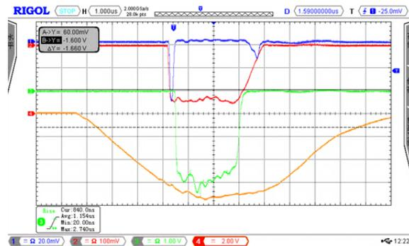
Figure 6: Incident wave (pink), reflected wave (blue), target current (green) and the voltage of electron gun(orange).
