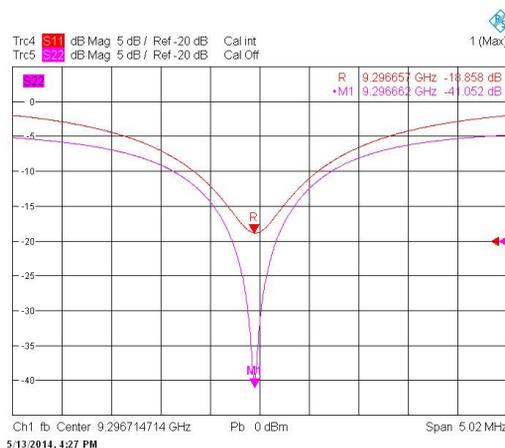
Figure 5: Frequency of the accelerating tube.
