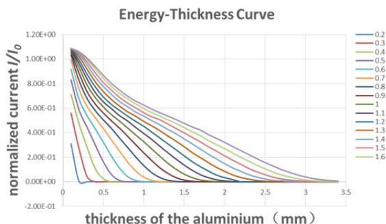
Figure 2: simulation data of the current ratio.
