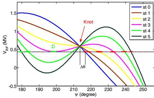
Figure 2: Twin RF bucket creation with synchrotron phase deviation. (From st 0 to st 5, the normalized RF voltages  $[\bar{V}_m, \bar{V}_h] / \bar{V}_m(0)$  is [1, 0.1], [1, 0.2], [1, 0.4], [1, 0.58], [1, 0.8] and [1, 1] respectively).
