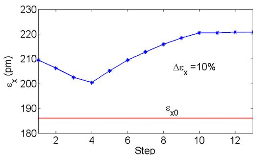
Figure 5: Equilibrium horizontal emittance during the injection process.
