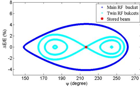
Figure 1: Twin RF buckets creation by two RF systems.
