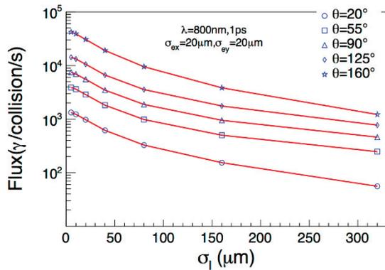
Figure 3: Flux of gamma ray changed caused by waist radius.
