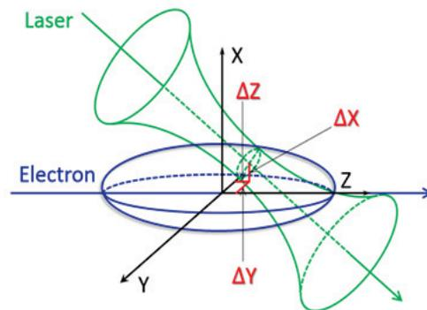
Figure 5: schematic diagram showing the deviation of laser waist centre from the centre of electron bunch.
