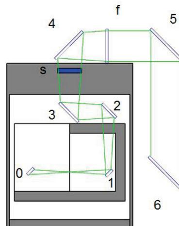
Figure 1: Basic optical structure (side view). The rectangles with number 0-6 represent plane mirrors, the rectangle referring to “f” is a convex lens, and the one with “s” is a transparent glass which covers the chamber.
