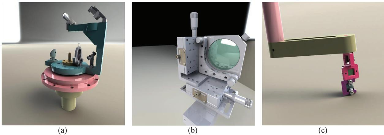
Figure 2: (a) Effect diagram of the rotatable bracket holding mirror No 0-3. (b) Translation device of convex. (c) Lifting bracket for fluorescent target.
