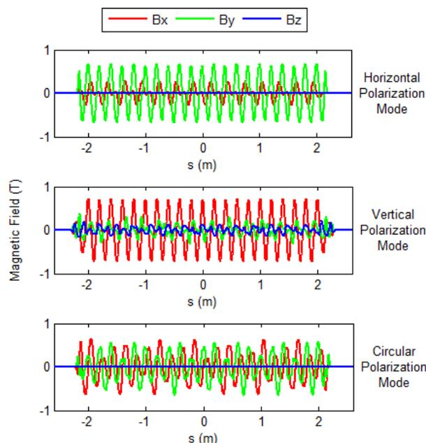
Figure 1: Magnetic field of the Knot-APPLE undulator at minimum gap.
