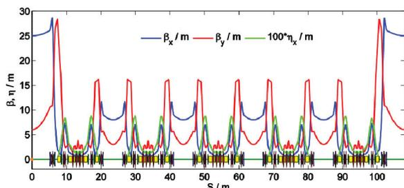
Figure 5: The Linear Optics of the SSRF-U Storage Ring
