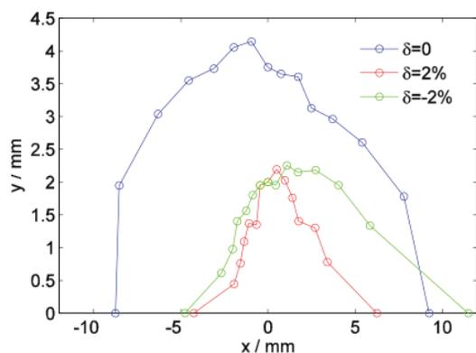
Figure 6: Dynamic aperture of the SSRF-U storage ring.
