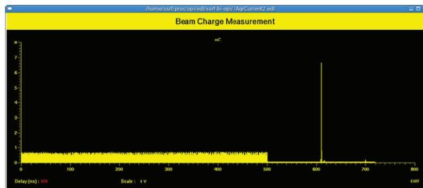
Figure 2: Hybrid bunch filling pattern in the storage ring.
