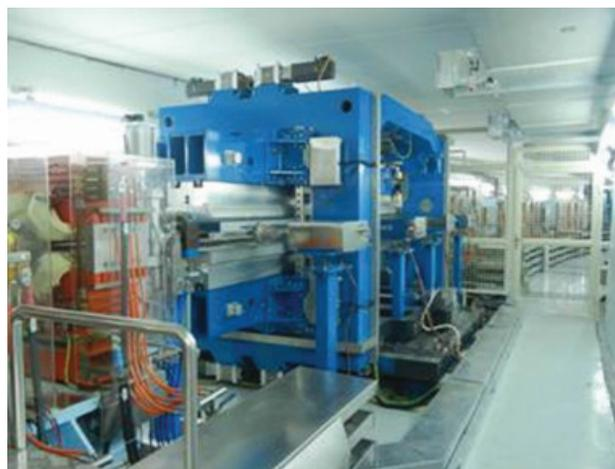
Figure 3: Twin EPU in the storage ring tunnel.
