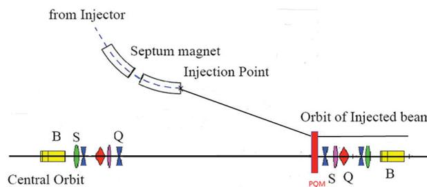
Figure 7: a new injection scheme for the SSRF-U.
