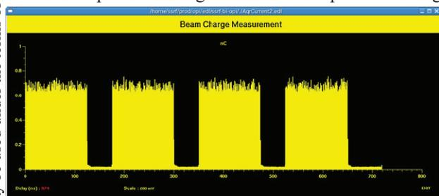
Figure 1: Bunch filling pattern of the SSRF storage ring.
