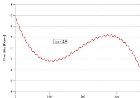
Figure 3: Calculated phase jitter when the undulator girder is deformed by 30 μm in parabolic shape. The girder is expected to be flat at the tuning gap and deforms when gap is changed from the tuning gap.
