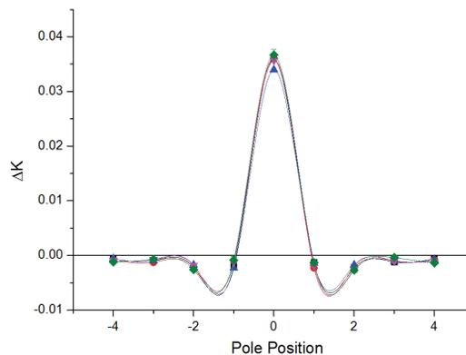
Figure 1: The measured local K changes due to a 100 μm pole correction at the 9.5 mm tuning gap. The abscissa denotes the distance to the pole: 0 is the tuned pole itself, ±1 the two next neighbouring poles etc.
