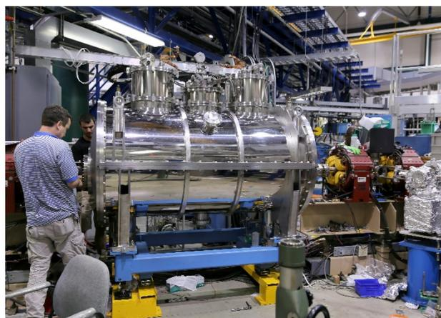
Figure 1: The MPW installed on the CAMD ring.
