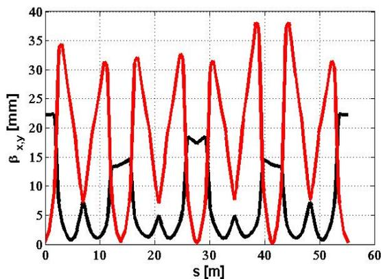
Figure 3: Betatron Function for CAMD with MPW at 7.5 T. Red = Vertical; Black = Horizontal.
