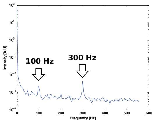
Figure 1: Tune jitter spectrum calculated from an acquisition of  $2.5 \times 10^5$  turns. Since a kick would not last enough to measure the low frequency components of the spectrum, we relied on the steady excitation from vertical instability to measure over a long period the betatron tune. For this purpose the vertical chromaticity has been reduced until the vertical instability was visible.
