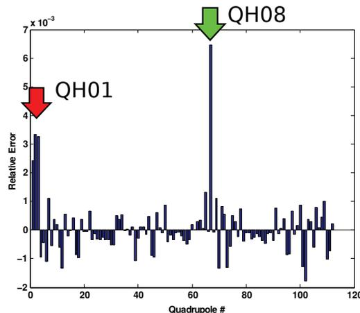
Figure 4: Quadrupoles errors reconstructed from turn-by-turn measurements in the Alba storage ring. The two arrows indicate the locations where the strength of two quadrupoles has been modified by 1%.
