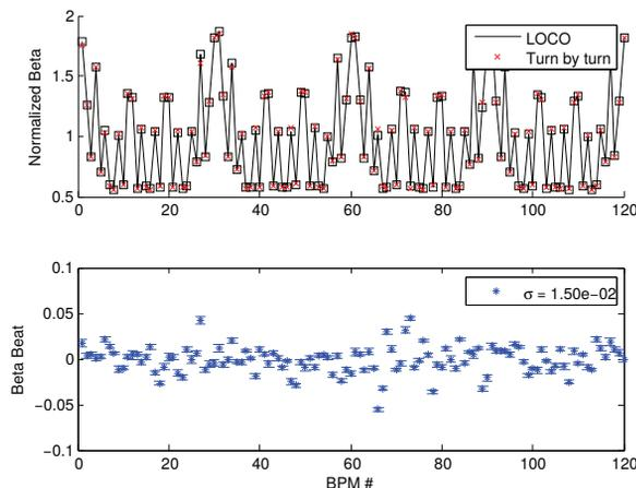
Figure 2: Top: Alba normalized horizontal betatron function from turn-by-turn measurements averaged over 100 kicks compared against the normalized betatron function estimated from LOCO. Bottom: Beta-beat and standard deviation. The error bars represent the reproducibility of the measurements, obtained from the standard deviation of the beta-beat over the 100 acquisitions
