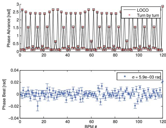
Figure 3: Top: Alba horizontal phase advance turn-by-turn measurements averaged over 100 kicks compared against the estimation from LOCO. Bottom: Phase beat and standard deviation. The error bars represent the reproducibility of the measurements, obtained from the standard deviation of the phase beat over the 100 acquisitions.
