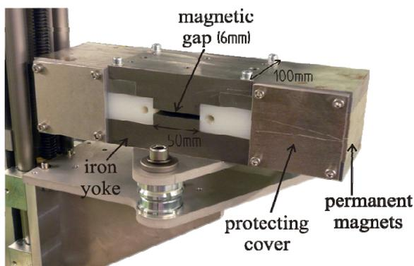
Figure 5: Reference dipolar magnet made at CELLS.
