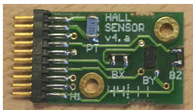
Figure 4: Hall probe head developed at CELLS.
